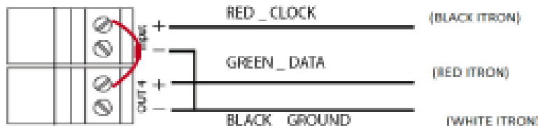
Figure 38: ORION Cellular LTE endpoint connection with resistor
